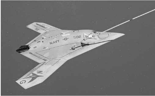
The Navy's unmanned X-47B receives fuel from an Omega K-707 tanker while operating in the Atlantic Test Ranges over the Chesapeake Bay. This test marked the first time an unmanned aircraft refueled in flight. U.S. Navy photo, April 22, 2015.
